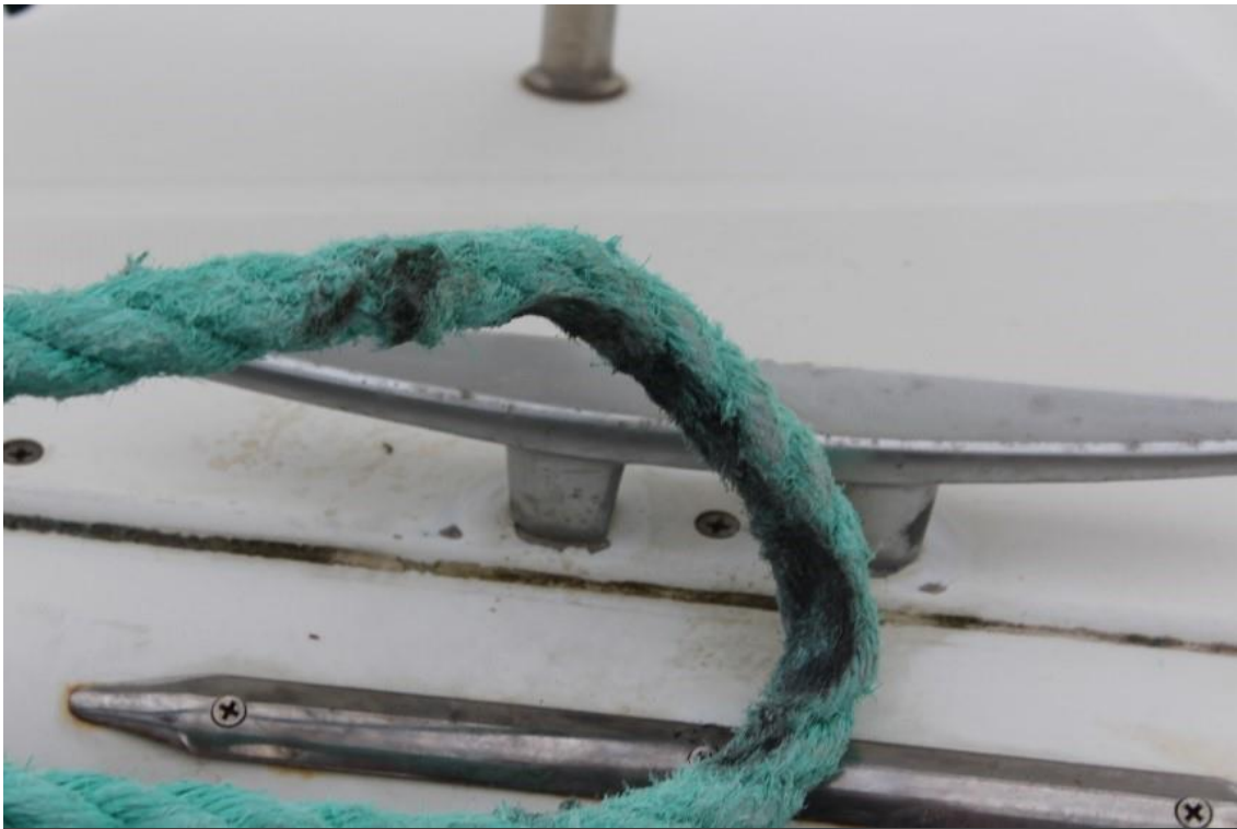
Mooring line showing wear caused by friction (heat) and compression.
