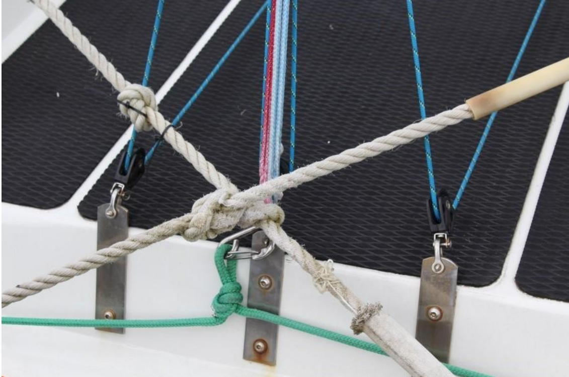
Knots in lines reduce strength.
