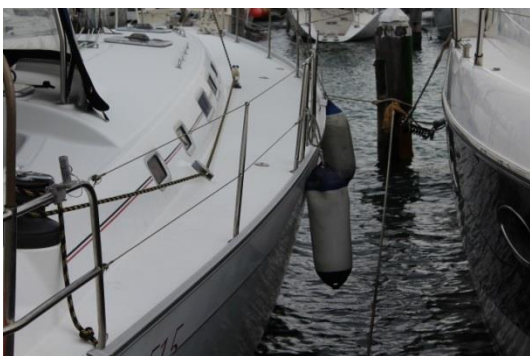
Fenders between vessels.
