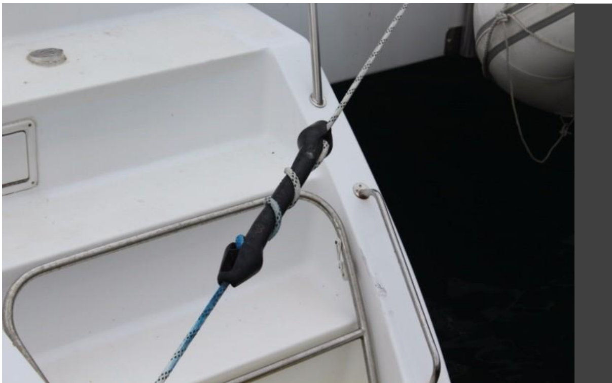
Mooring compensator absorbs shock loads caused by wave action
