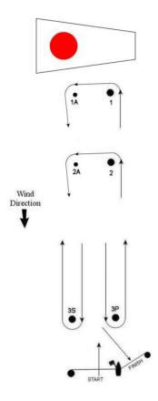
If one of the gate marks (3S or 3P) is missing, boats shall leave the remaining mark to PORT
