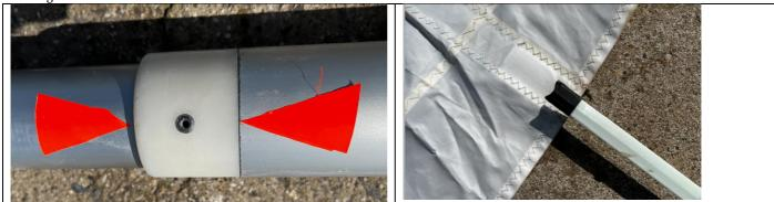
**C** Fit rudder with tiller **under** the traveler, fit gudgeon R clip and fit transom bung.
