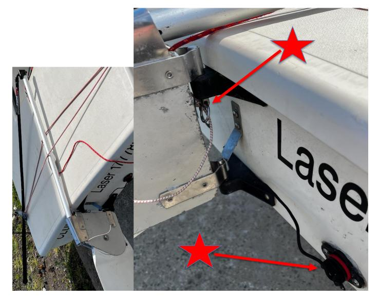
**D** Step mast and fit the mast retention shock cord to the gooseneck with the small stainless steel hook.
