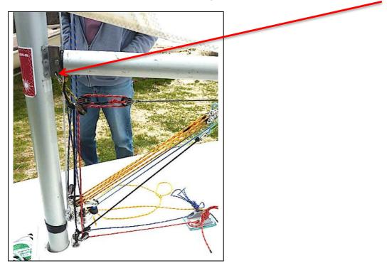
**Outhaul** Take the grey dyneema line of the outhaul a. thread through the fairlead at the end of the boom, b. through the clew of the sail c. pass the loop over the end of the boom and d. Fasten the clew strap – tight enough for the sail to just touch the boom but not too tight!
