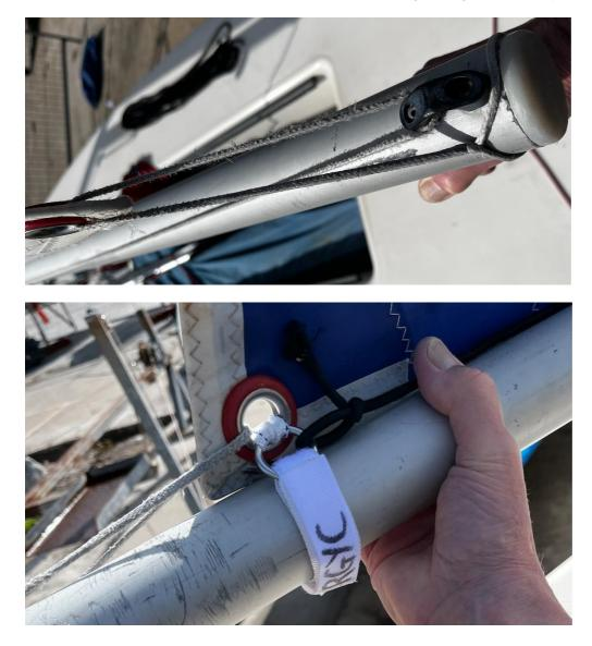
**F** Vang. Attach the vang with the pin and clip to the vang tang on the mast. Press down the boom and attach the vang key to the boom. Tie the tail of the yellow control line to the front corner of the centreboard.
