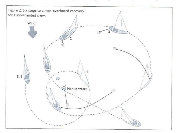
2. The Lifesling is deployed by opening the bag on the stern pulpit and dropping the sling into the water. It will trail astern and draw out the line.
