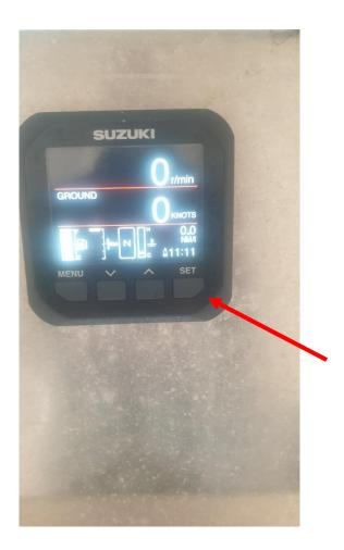
Turn the ignition on, press the set button to get the display that shows Fuel, RPM, Speed, Trim and Temp
