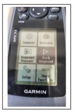
An **Optional step** is to rename the waypoint by moving the cursor to the screen and pressing "Select" then editing the name by using the cursor and select.
